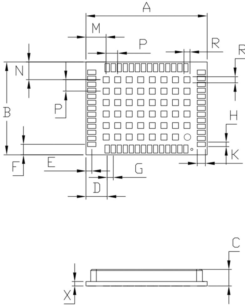
**Figure 2-2 UM980 Mechanical Dimensions**
