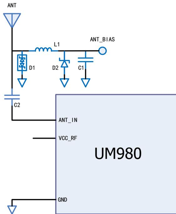
Figure 3-2 UM980 External Antenna Feed Reference Circuit
